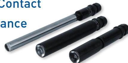
FDR-800 Series Probes provide optimum performance in the non-contact analysis of powders and other diffusely reflecting materials. They feature, large depths of field, adjustable sample offset distance, and low stray light. Specialized models are available for in-situ self-cleaning (FDR-825).
