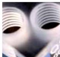
Thanks to its two optical path lengths and the innovative internal thread cut directly in the quartz glass cuvette.
