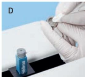
D Clean window and cap (TrayCell remains in spectrophotometer).
