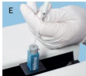
E Pipette new sample onto window.
