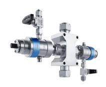
The Hellma Excalibur HD FCP transmission cell brings high performance chemical composition monitoring to a wide range of demanding applications – in the process or in the pilot plant. The sampling interface consists of two standard optical fingers combined with either off-the shelf Swagelok components or the highly precise H-Cell central part.
