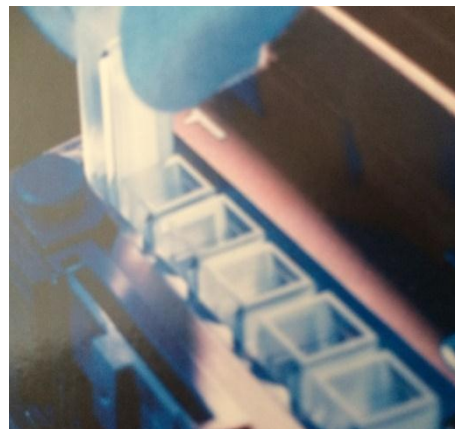
The holder positions the cuvette in the light beam
