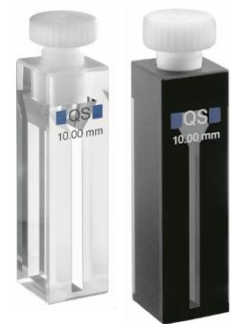
Non-masking and self-masking cuvettes
